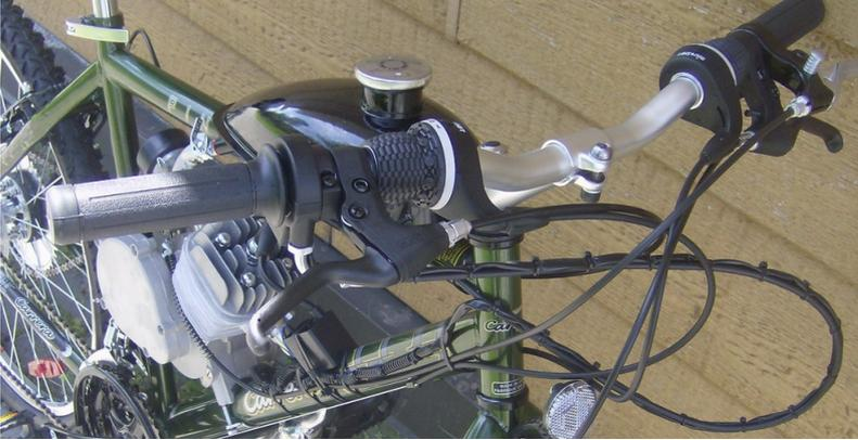
Remove existing right handle grip and replace with twist throttle.
