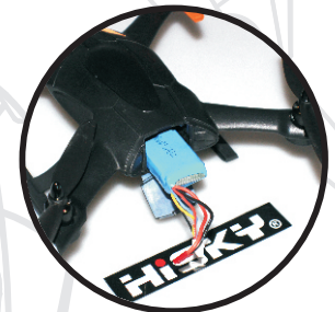
Step 4: Take out the battery of the quad
