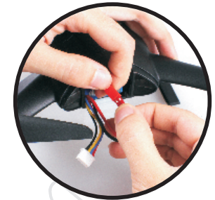
Step 2: Disconnect the battery
