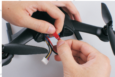
Step 2 connect the battery of the model with the main board.
