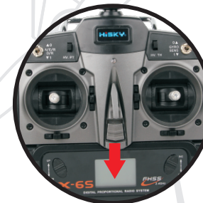
Step 3: turn off the transmitter
