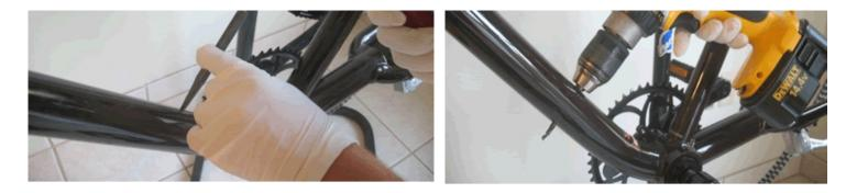
The longer bolt goes through the bike frame then through the motor mount) As shown on photos below:
