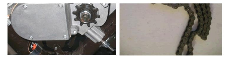
Install chain guide pulley. Do not over-tension the chain. Install chain guard and replace spark plug
