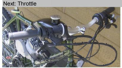
Remove existing right handle grip and replace with twist throttle. Existing brake lever loosen and shifted to facilitate installation of twist throttle Replace brake lever in its original position after installation of the twist throttle
